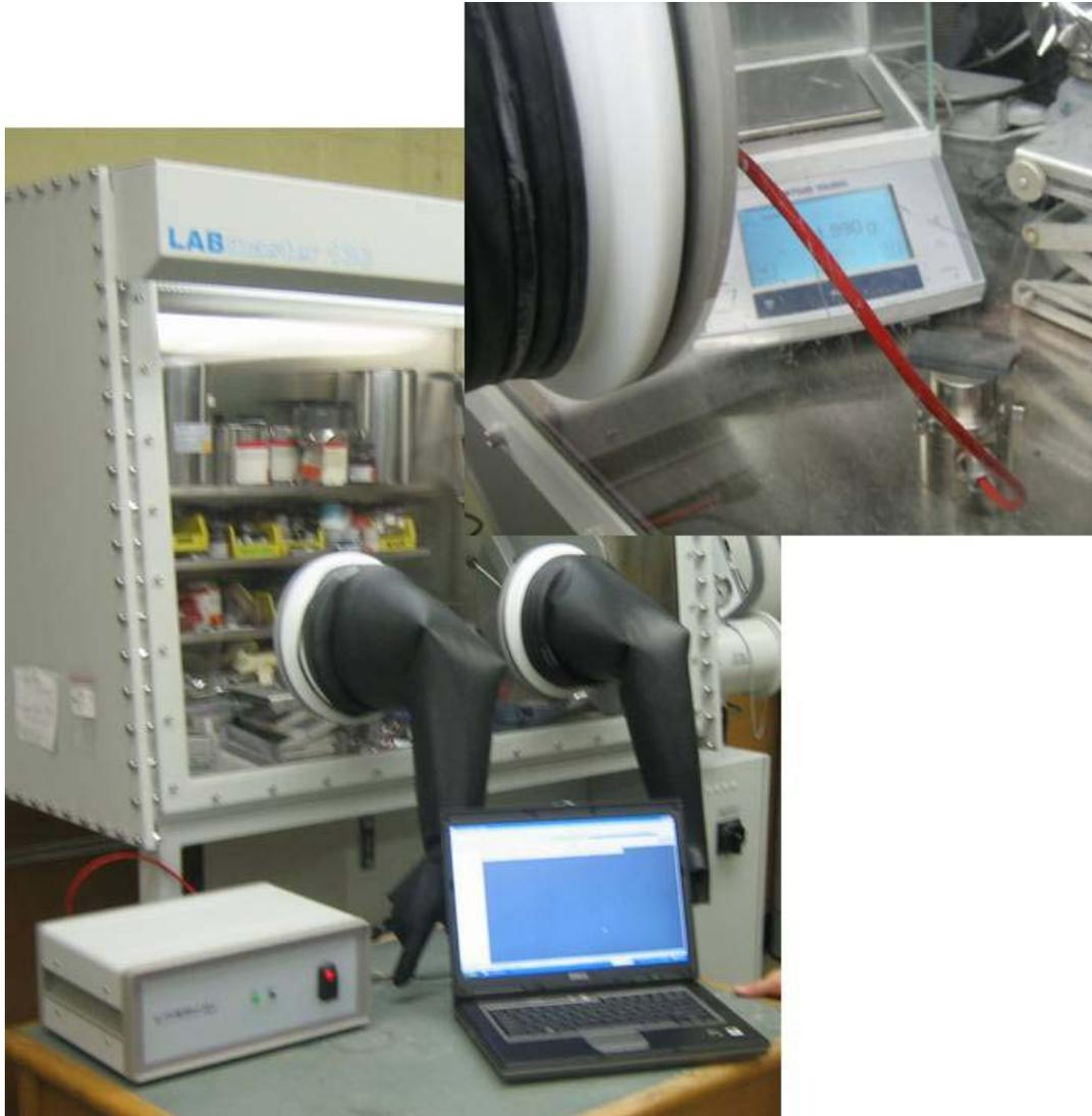
Figure 2 – Images of C-Therm's probe being used inside a glove Box
