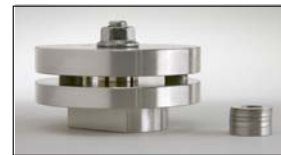
Compression Set Rig EV 03 , according to ISO 815-1.
