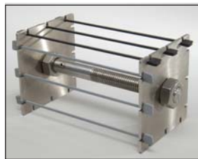
Tension Set Rig EV 04 , according to ISO 2285.
