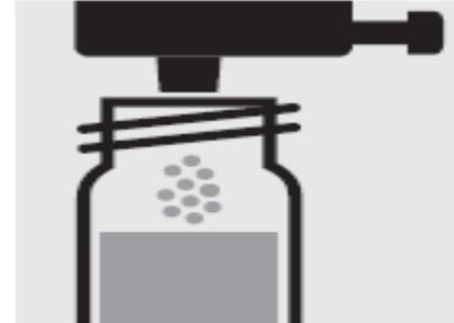
Add 1 dose of  $\text{NH}_4\text{-1K}$  using the blue dose-metering cap, close the cell with the screw cap.
