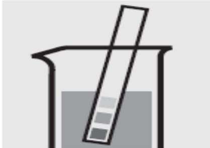
Check the pH of the sample, specified range: pH 4 – 13.
